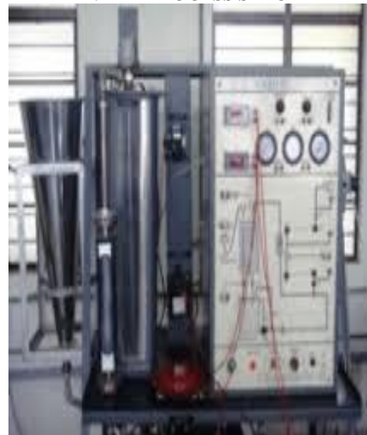
Fig 2 Level Process Station
